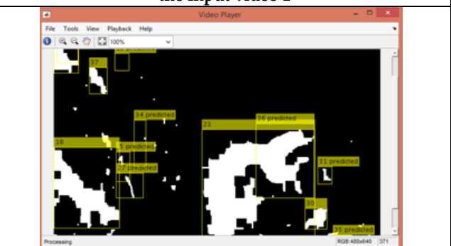
Figure 8: Frame extraction for the detected objects in the input video3
